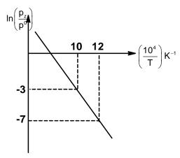
$$(1) \Rightarrow ln\left(\frac{p_z}{p^0}\right) = -\left(\frac{\Delta H^0}{10^4 R}\right) \times \frac{10^4}{T} + \frac{\Delta S^0}{T} \dots (2)$$
